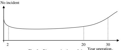
Fig. 3. Changes in time of the transformer damage
